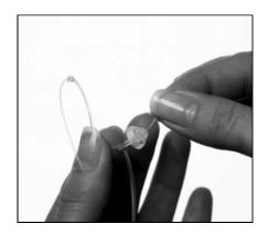
Avoid taking the dome and the slimtube apart regularly as this weakens the connection. The tube and dome would then be more likely to separate inside your ear.
